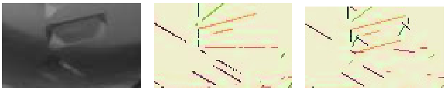
Fig. 5. Left: zoom over original image in Fig. 2. Center: segment detection results by the pseudocolor fuzzy Hough transform. Right: results of segment detection through the proposed segment detector.
