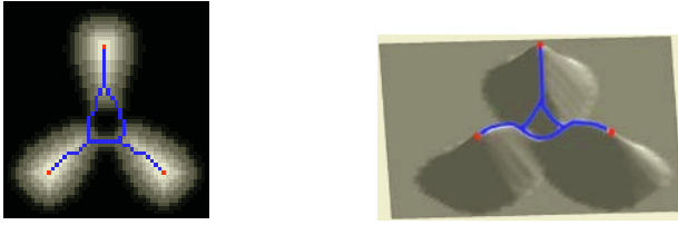
Fig. 2. Left: A synthetic 2D grey-level image. Right: Grey-level landscape. MGR and local maxima are overlaid (blue and red, respectively, in the electronic version of the paper).
