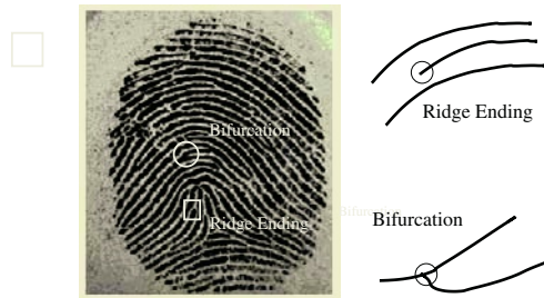
Fig. 1. A minutiae feature (a ridge ending and a bifurcation) in a fingerprint image.
